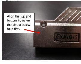
Once the three holes are properly aligned, the cover top and bottom assembly screws can be torqued. (Torque 4.7 ~ 5.5 inch/lbs)
