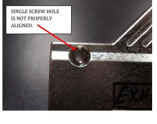
Ensure the holes are properly aligned before torquing down the screws. We recommend you start the single screw first to ensure proper alignment.
