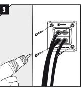
EzEntry<sup>™</sup> 4 mini is compressed and sealed when you tighten the screws.
