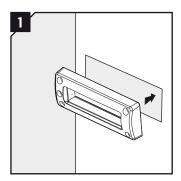
Insert the frame into the opening.
