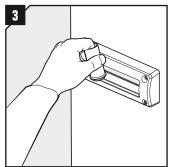
Lubricate the inside surfaces of the frame with Roxtec Lubricant. Make sure to lubricate the corners.
