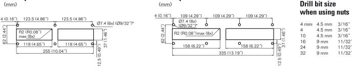
Cut a rectangular opening for the frame, according to the dimensions above. \* Recommended drill bit size.
