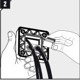
Insert all modules from the back of the frame and install all cables before attaching the frame to the structure.
