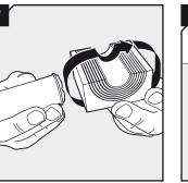
Lubricate all modules thoroughly, both on the inside and the outside surfaces, before installation.
