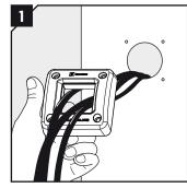
Lubricate the inside of the frame and the modules with Roxtec Assembly Gel. Feed the cables through the frame.
