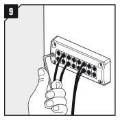
Tighten the integrated compression unit with a hex key to seal the transit.\*
