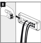
Insert the modules according to the installation plan (Packing plan).
