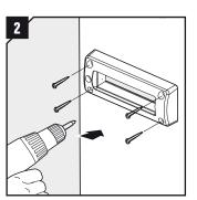
Attach the frame firmly, using the enclosed screws.
