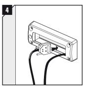
Feed the cables through the frame opening.
