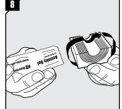
Lubricate all modules thoroughly, both on the inside and the outside surfaces, before installation.
