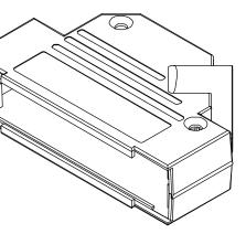
CONNECTOR COVER 1. MATERIAL: Zinc die-cast 2. FINISH: nickel over copper under-plate
